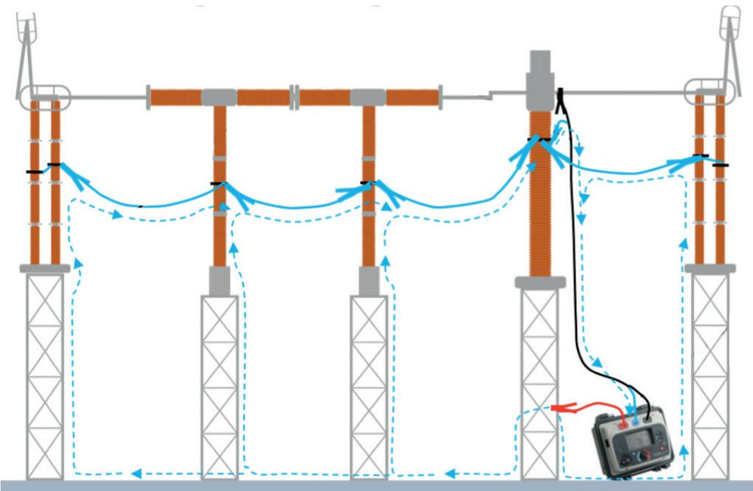
GILS kit in use to guard against surface leakage disrupting the measurement.
