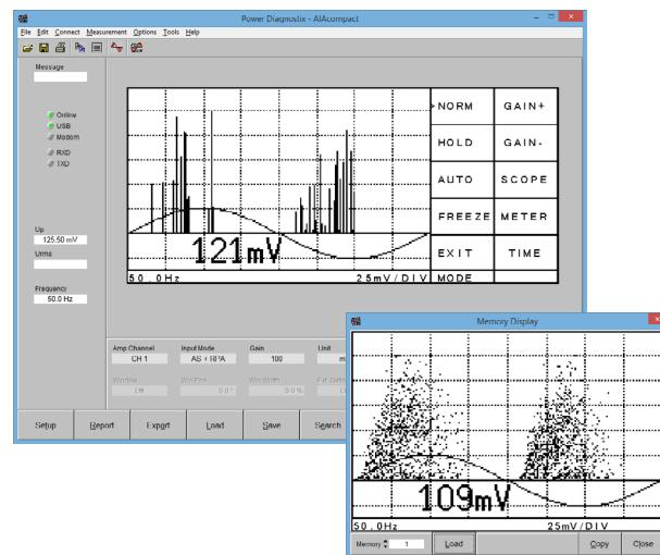
The ten menu buttons on the LCD can be used in the same manner as the physical ones on the instrument. These allow the unit to be controlled remotely, even over long distances. Additionally, the software allows the acquisition of coloured PD patterns that show more in-depth information than black and white patterns. These patterns can then be exported as bitmap files.
