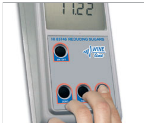
3 Press READ and View the Results on the LCD
