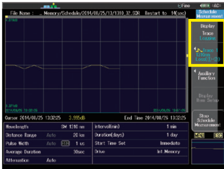
Example of logging the loss value between markers ① and ②
