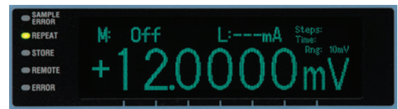
High resolution output with \pm 120000 display counts and 100 nV steps minimum
