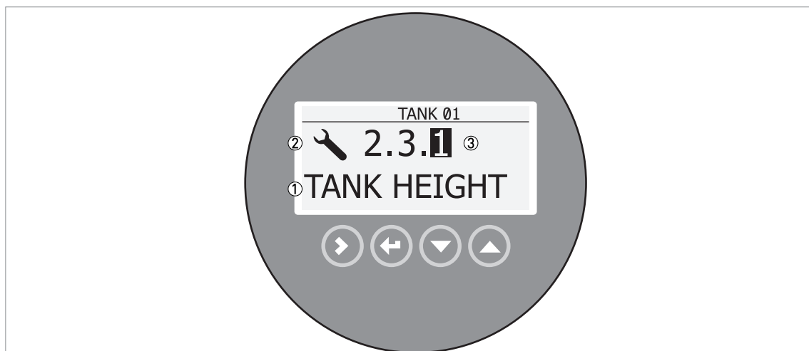
Figure 5-2: Local display screen layout in configuration mode
