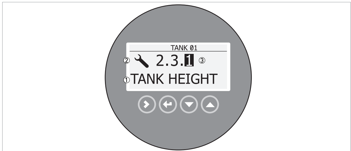
Figure 6-1: Local display screen layout in configuration mode
