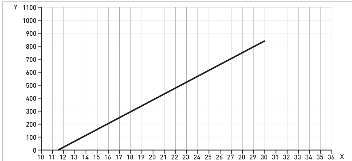
Figure 8-2: Minimum power supply voltage for an output of 22 mA at the terminals (Non-Ex and Hazardous Location approval (Ex i / IS))
