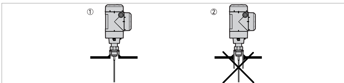
Figure 3-9: Sockets for threaded process connections
