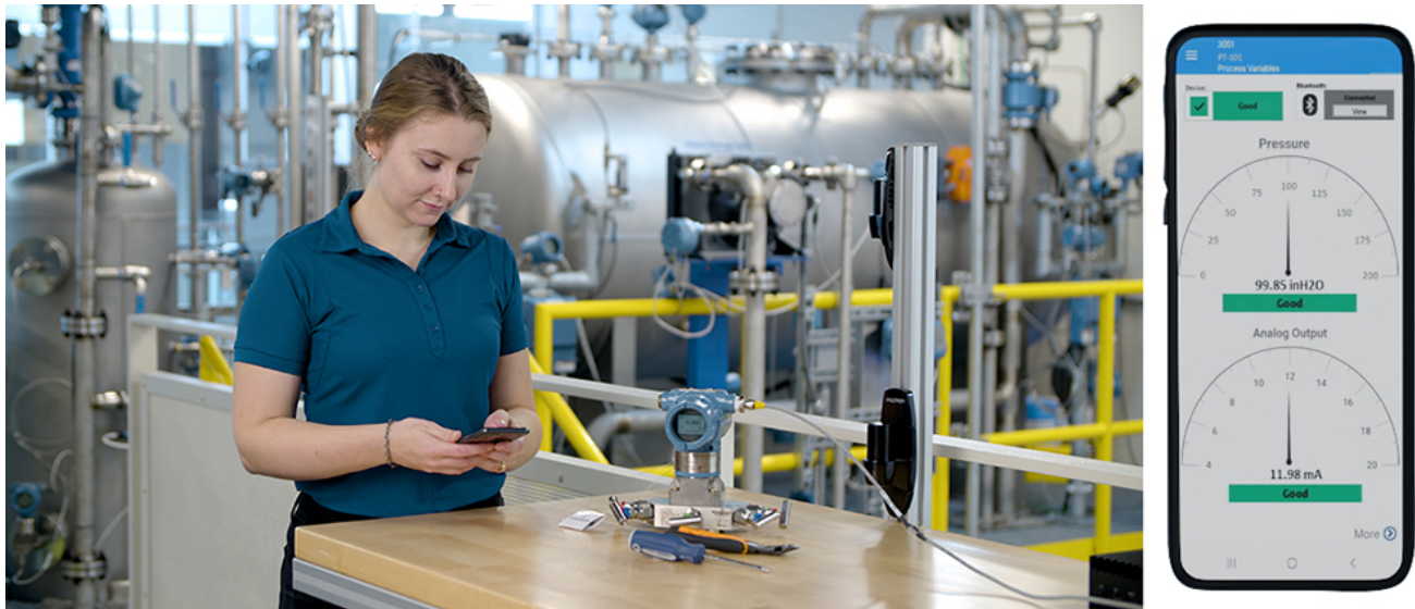
FIG. 4. New configuration tools designed for Bluetooth technology use the same interface as HART communication, so experienced technicians will find them very familiar.
